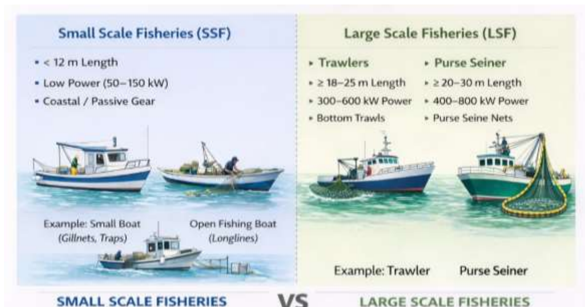
Figure 1. GFCM classification of fishing vessels
